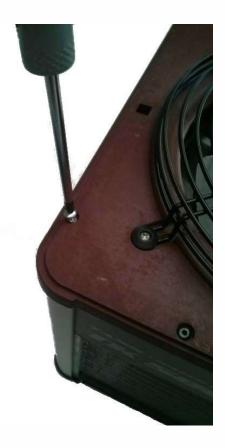
Using the screw-driver, remove the 4 INOX screws indicated in the picture here below.
