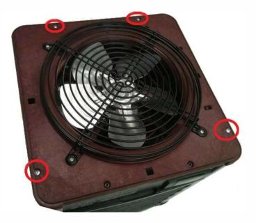
Remove the red fan support lifting it up from the bottom edge. Leave it on the metal cover, as you can see in the picture.
