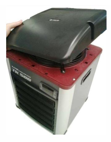
Remove the conveyor from the top part of the chiller. You can see the metal black grid and the red fan support.
